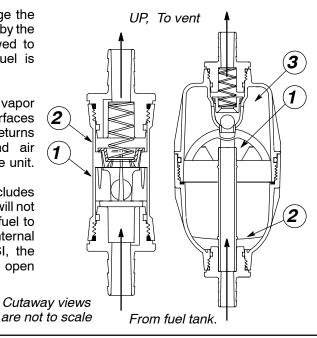
**LG100:** 1. In the First Stage the venting tank fuel is deflected by the Flow Diverter. Fuel is directed down to the drain ports and air is allowed to bypass and continue traveling up.
